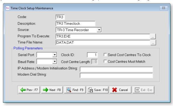
**Serial Port** The Serial Port is a 9 or 25-pin socket on the back of your computer into which the Time Clock data cable (serial cable) is plugged. Entering on this field will display a list of Serial Port options. Usually it would be Com1 or Com2.
