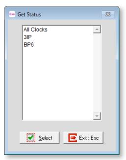
Select a timeclock from the list in order to query the status of the hardware connection, i.e. the data cable and/or modems, that link your computer with the electronic timeclock. Alternatively, select **All Clocks** to query the status of all clocks. A Timeclock Status report that is free of errors indicates a successful connection:
